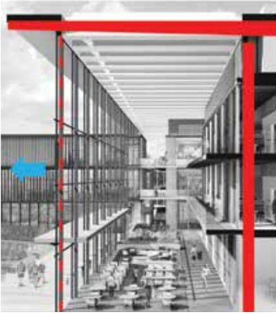
Schematic section at Commons showing the framing geometry of the column (right), glass wall (left) and the roof cantilevers (top).
